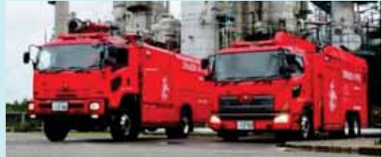
Core vehicles of the Dragon Hyper Command Units Hose extension vehicle equipped with large water cannon (left) Large-capacity water pump vehicle (right)
