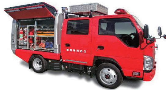
Small vehicle loaded with rescue supplies and equipment and equipped with a power pump
