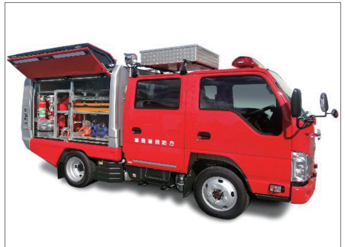
Vehicle equipped with small mounted powered pump and rescue equipment (Measures regarding volunteer fire corps which form the core of regional disaster prevention capabilities)
