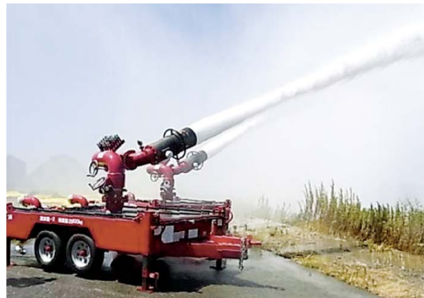
Water spraying drill using a high capacity foam system (Osaka/Wakayama wide-area joint disaster prevention council)
