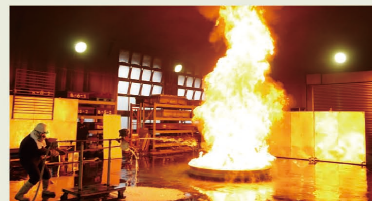
ISO規格 低発泡B火災試験 Class B fire test of ISO standard for low-expansion foam
