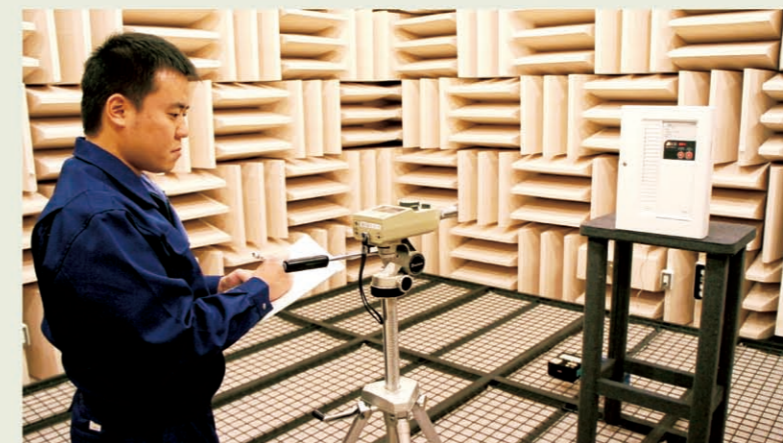
受信機の音圧試験 Acoustic pressure tests of control & indicating equipment
