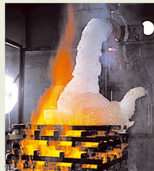
高発泡A火災消火試験 Class A fire test with high-expansion foam
