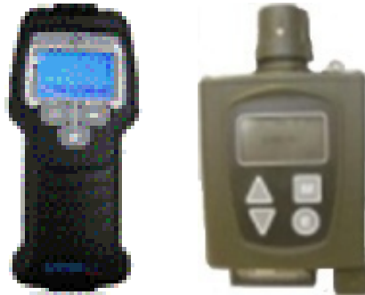
Chemical Agent Detector (nerve agent, blister agent, blood agent and choking agent)
