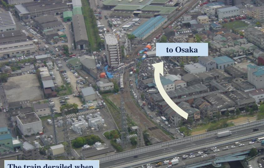
The train derailed when running on right hand curve – R304m
